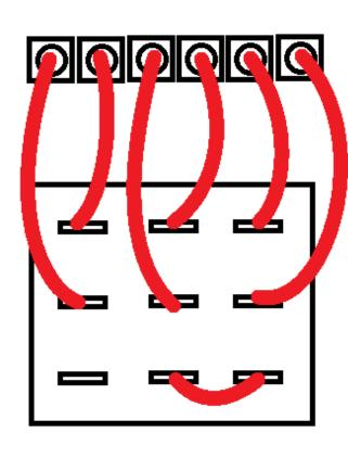
If you prefer to solder the 3PDT directly to the board, you can wire it as shown in the schematic. We recommend to use the **provided 3PDT PCB adapter** to make the soldering easier.
