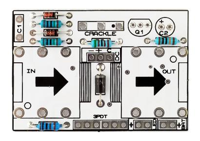
Place the resistors and diodes. If you have troubles reading the values, check out our "Reading Part Values" tutorial.
