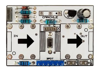
Solder the capacitors and transistors. If you have troubles reading the values, check out our <u>"Reading Part Values"</u> tutorial. Pay attention to the orientation, as well as to the polarity for electrolytic capacitors.
